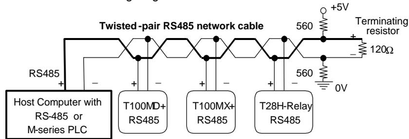
Since there is only a single pair of wires that are connected to all the RS485s, the same two wires will thus have to carry the serial data input to the each device as well as the serial data output from the device.
